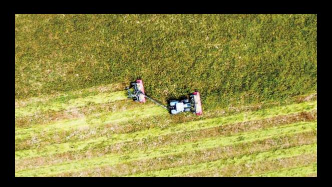
With a full-width baffle mounted to the conditioner and protective forming shields that can be adjusted to a narrow 5-foot (1.5 m) opening, the R1 FR is ready to lay down well-formed, tailored windrows to meet your needs.
