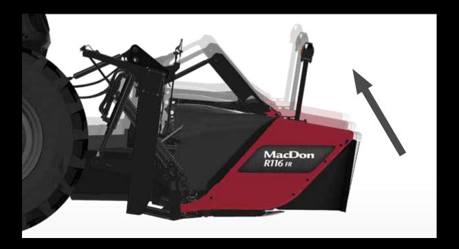
Using minimal ground pressure, the R1 FR's Responsive Float System moves the unit "up and back" as it encounters bumps in the field. This dynamic movement results in true ground following and helps ensure a clean, even cut of your fields.
