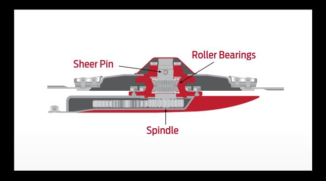
Each disc spindle on the R1 FR Series cutterbar features a shear pin designed to shear if it comes in contact with a large object in the field. Once sheared, the disc moves up and out of the way of the other discs, reducing the risk of severe damage to the cutterbar. Operators can replace shear in-field and get back to mowing in a short time.
