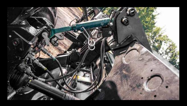
The three-point hitch on MacDon's Front Mount Rotary Disc unit is compatible with category 2, 3, and 3N tractors. Cutting disc runs at 2652 rpm @ 1000 PTO; a PTO Completion Package is required and installed by your MacDon dealer.
